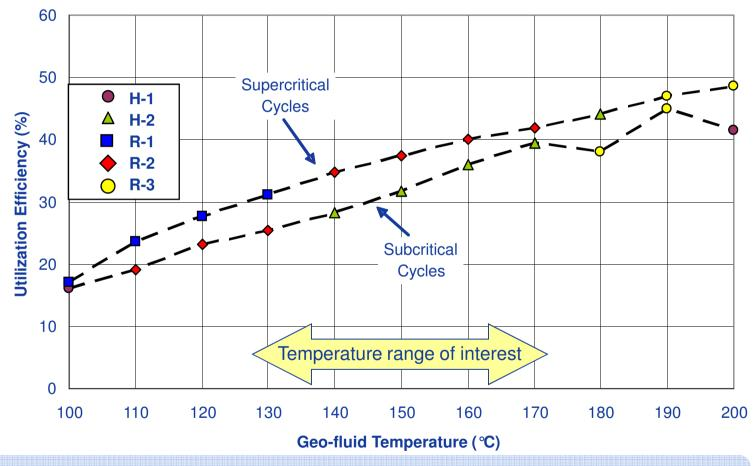
Supercritical cycles provide higher utilization efficiency for all geo-fluid temperature range, resulting in max 23% increase in net power.
